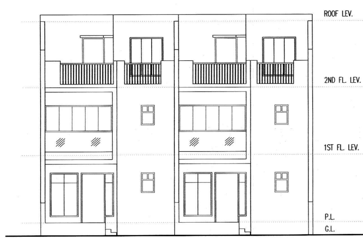
RESIDENTIAL BUILDING (BUNGLOW) FRONT ELEVATION SCALE-1:100
